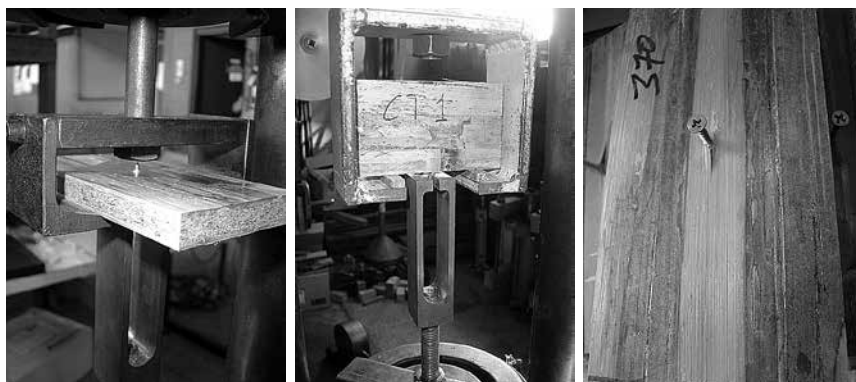
Figure 14 – Screw pullout strength test (reinforced boards).
