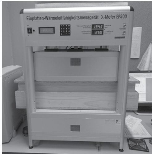
Figure 3 – Guarded hot plate \lambda -Meter used in the thermal conductivity tests.
