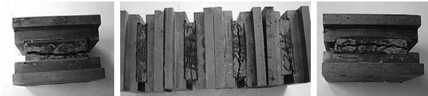
Figure 13 – Aspect of the specimens after the internal adhesion tests.
