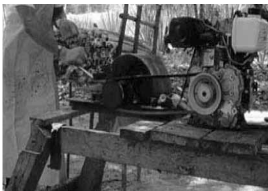
Figure 1 – Shredding Machine called “Tapuia” used on the production of curauá fiber.
