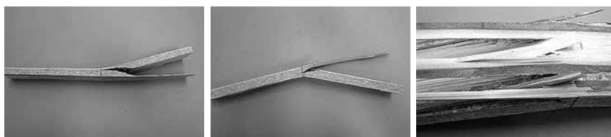
Figure 12 – Detachment of the reinforcement after the static bending test.
