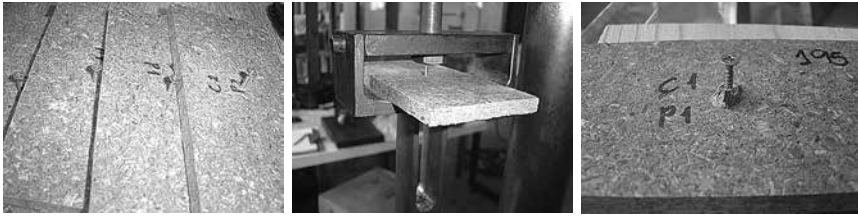
Figure 15 – Screw pullout strength test (unreinforced boards).
