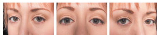
FIGURE 1.3 The relative position of the pupil and corneal reflection does not change when the head moves but the person is looking at the same spot.
