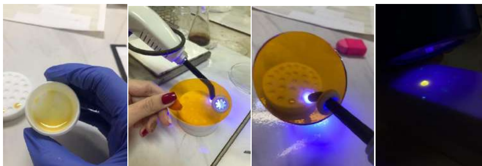
Figure 01. Photopolymerization using pyrrole-pyrroles and UDMA, BIS-DMA and TEG-DMA.
