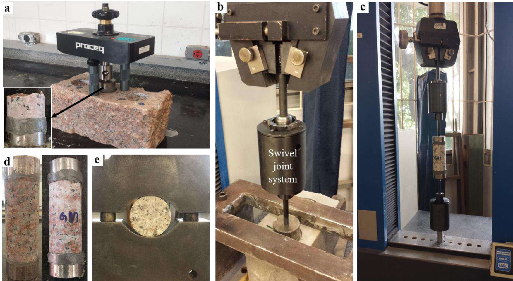
Fig. 2.2. a. POT with the DY-216 device; b. POT with the Emic DL-10000™; c. DTT in progress; d. DTT specimen preparation and e. BDT according to ISRM (ISRM 1978).
