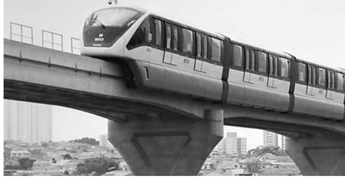
Figure 1 Straddle-type monorail vehicle
