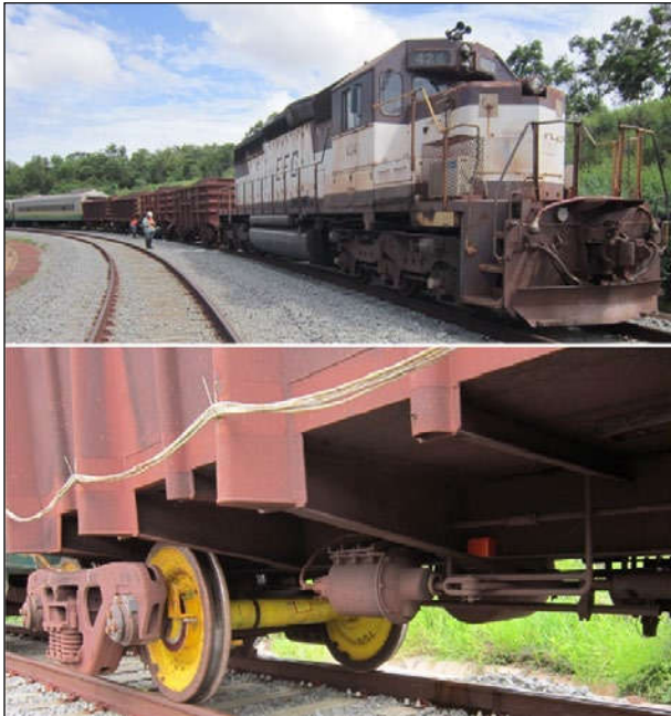
Figure 5 – Train - IWS (yellow) and IMU(red)
