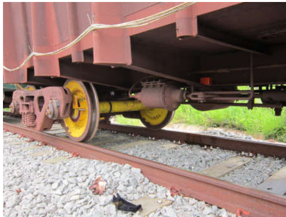
INSTRUMENTED WHEELSET AXLE BOX ACCELEROMETERS
