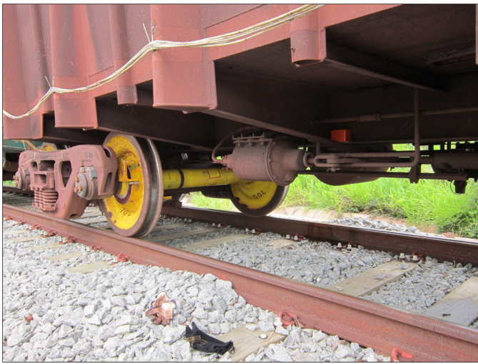
Fig. 6. Instrumented wheelsets and measuring system (image by the author)
