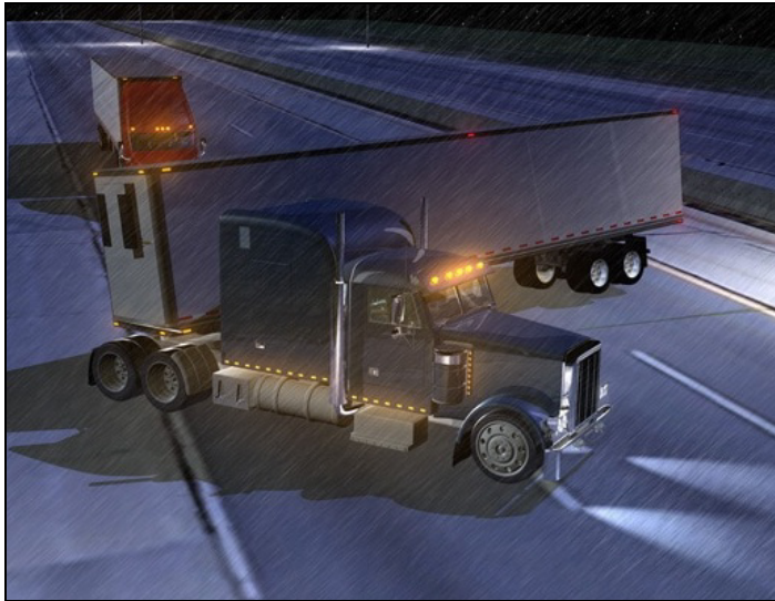
Figure 1 Truck/semitrailer jackknifing (Art from AS in internet) (see online version for colours)
