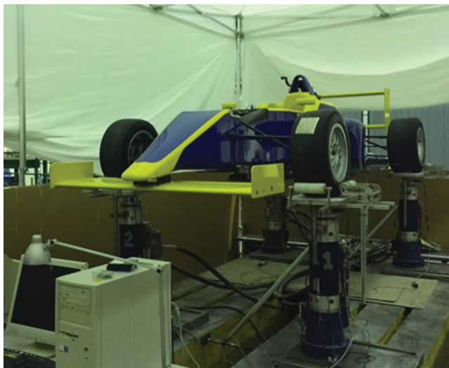
Figure 1. Real vehicle on the Four Poster rig.
