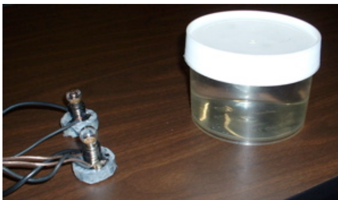
Figure TG1-8: Alternative, inexpensive cylindrical lens—a smooth-walled plastic jar filled with water.
