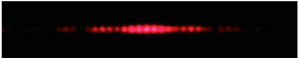
Figure TG3-4 Photo of fringe pattern produced by laser light shone on two narrow slits separated by a small distance.
