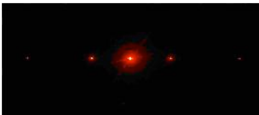
Figure TG3-5: Photo of fringe pattern produced by laser light shone on a diffraction grating.
