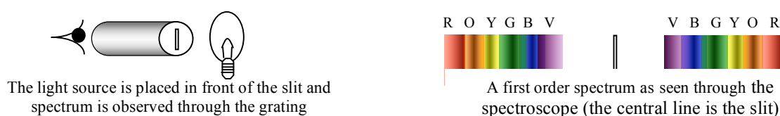
Figure TG4-3: Spectrum of white light as viewed with the simple spectroscope.
